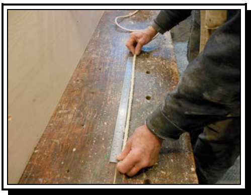
Cut rope to 21 in. (6 pieces)
