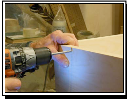
Drill through existing hole into the cleat inside
