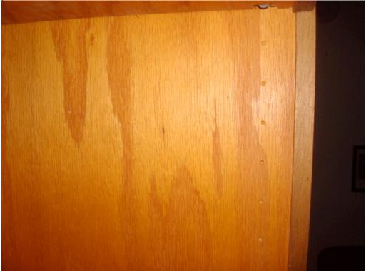
Then I drill a 3/8" hole 5/16" deep right in the edge of the underside of each shelf so that a 3/4" #8 pan head screw driven into the hole so about 1/4" protrudes. When the shelf is put in place the viewer can't see the screw. When getting the bookcase ready to use as a coffin, the shelves and screws are readily removed and the holes are not noticeable.
