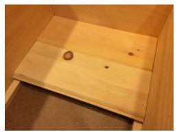
Turn coffin right side up. Place bottom boards on cleat, fitting tongue into groove as you go.
