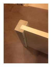
Insert edge of end boards into groove. If you are using the square spruce pieces, see the photo below.
