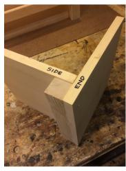
Option: Screw end boards to 1½"x1½" aligning the end of the boards and the edge of the corner board.
