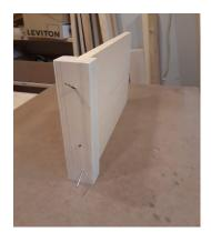
Attach end to corner with 2" Fin-Trim screws driven in at an angle. Assemble both end pieces.
