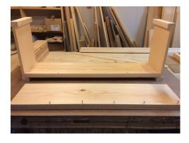
Attach 3/4" x3/4" cleat along bottom edge, spacing 1 1/4" screws every 8" (pre-drill 1/8"holes for screws in the cleat). Flip coffin over and attach other side and cleat.
