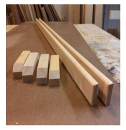
Cut an angle off two corners of the handle supports. Put two of them on the side of the coffin so that they span any joint between side boards and are spaced evenly between the ends. Outline the location with a pencil, drill screw holes, then attach the supports with 2" screws driven from the inside of the coffin.
