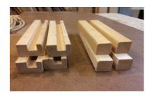
Cut corner boards to inside depth plus  $1\frac{1}{2}$ ", then cut a  $\frac{3}{4}$ "x  $\frac{3}{4}$ " groove  $\frac{1}{2}$ " in from the long edge using table saw or router.
