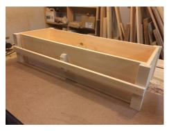
Round the edges of the handle boards so the coffin may be carried comfortably. Screw handles to corner boards and supports using 2" screws.
