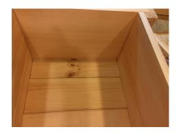
You will probably have to cut the last board to fit into place. Then put the other 74"cleats on top of the bottom boards and screw the cleats to the coffin side.
