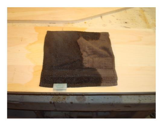
On the kerf side of the board, pour boiling water in the kerfs, then turn the board over. Spread a hand towel on the board and pour boiling water on the towel. Leave the towel in place for a minute or so, pouring a little more water on the towel to keep the temperature up. Alternatively, you can use an iron on the wet towel to heat the wood.
