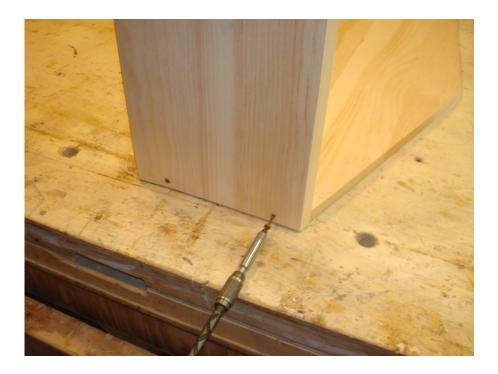
Saw the two end pieces to length and width (the grain runs vertically, so the length is the width of the side boards), attach the two end pieces to the bottom board and plane the edges to match the bottom.
