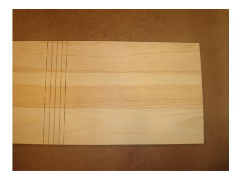
Saw the two side boards to width, the depth of the body plus one and one half inches, then mark the location of the shoulder on the side boards. Draw a pencil line across the boards from that shoulder line, then draw two lines on each side of that line spaced three-quarters of an inch apart, five lines in all.
