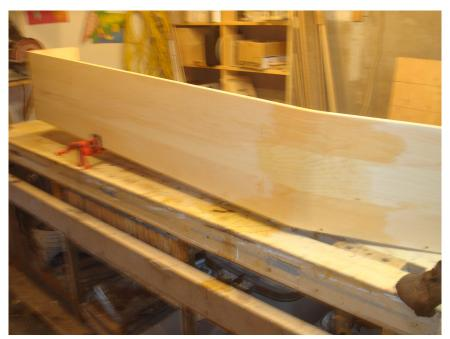
Gently bend the lower part of the side board around the shoulder curve, then use a clamp to hold it in place against the edge of the bottom board. Drive screws through the pre-drilled holes into the edge of the bottom board. Check to see that the end pieces are perpendicular to the bottom board and screw the side boards to the end pieces.
