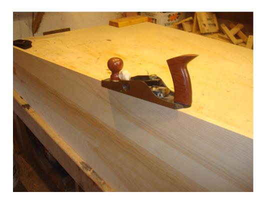
Saw just outside the pencil lines, then plane the edges smooth and form the shoulders into a gentle curve.
