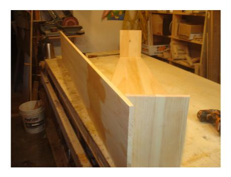
Set the bottom-plus-ends assembly on the workbench, position the side board so the kerf is centered on the shoulder curve, then put two screws in the bottom edge of the side board on the side toward the top of the coffin and drive them into the edge of the bottom board.
