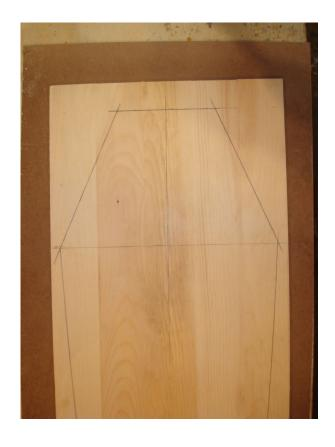
Lay out the coffin bottom on a board, adding two inches to the length and two inches to the width at the shoulder (the shoulder line is about 14 inches from the head end of the coffin). The head end is nine inches wide and the foot end eleven inches.
